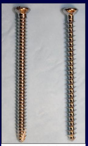
Figure 1: Four-mm outer-diameter cortical (left)
