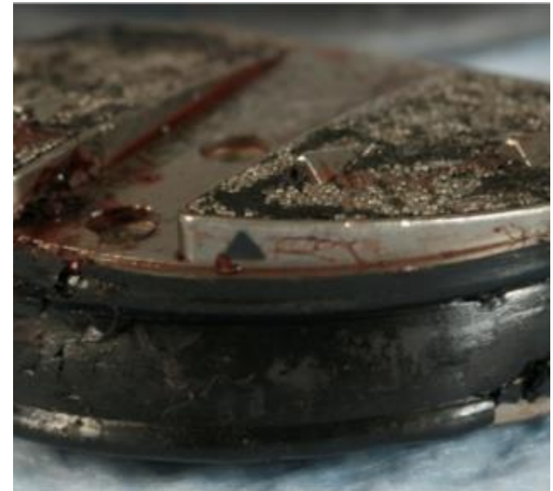
Figure 4. Failed acetabial cup.
