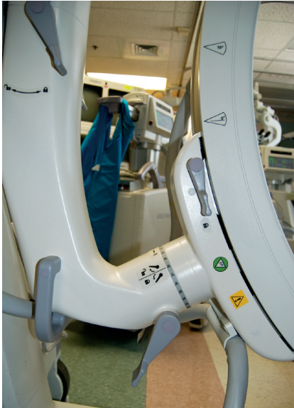
Figure 9. Example of the brake handles and lock indicators on a mobile fluoroscopy unit.
