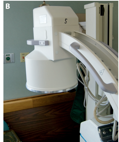
Figure 5. A. Diagram of an image intensifier used in a mobile fluoroscopy system. B. The image intensifier of a mobile fluoroscopy unit. The image intensifier increases the brightness of the fluoroscopic image.
