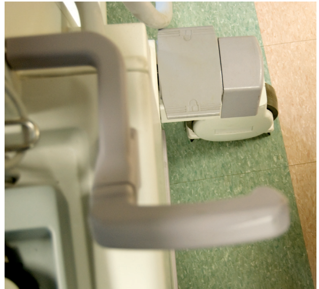
Figure 13. The handles on a C-arm help steer the base of the unit. Note how the handle and wheel are turned in the same direction. Also note the pedal brake associated with the wheel.
