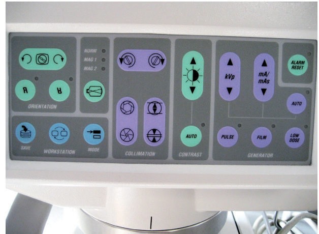
Figure 2. Above. Mobile fluoroscopy control panel. This control panel is separated into 5 different categories: orientation, collimation, contrast, generator and workstation.
