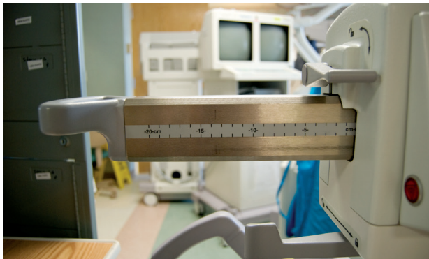
Figure 12. The C-arm can move forward and backward in relation to the base of the unit, a feature called telescoping.
