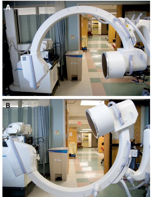
Figure 10. During orbital rotation, the x-ray tube and image intensifier or flat panel detector glide along the natural curve of the C arm. A. Overscan. B. Underscan.
