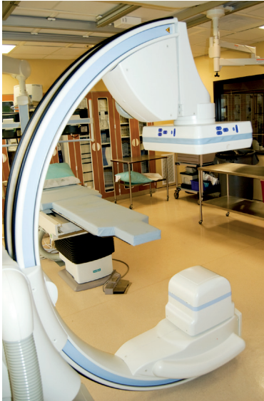
Figure 6. Flat panel detector. The flat panel detector may one day replace the image intensifier as the standard image receptor in the mobile fluoroscopic system.
