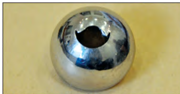
Figure. Metal hip prosthesis causing cobalt intoxication. Removed metal head with hole due to severe metal loss.
